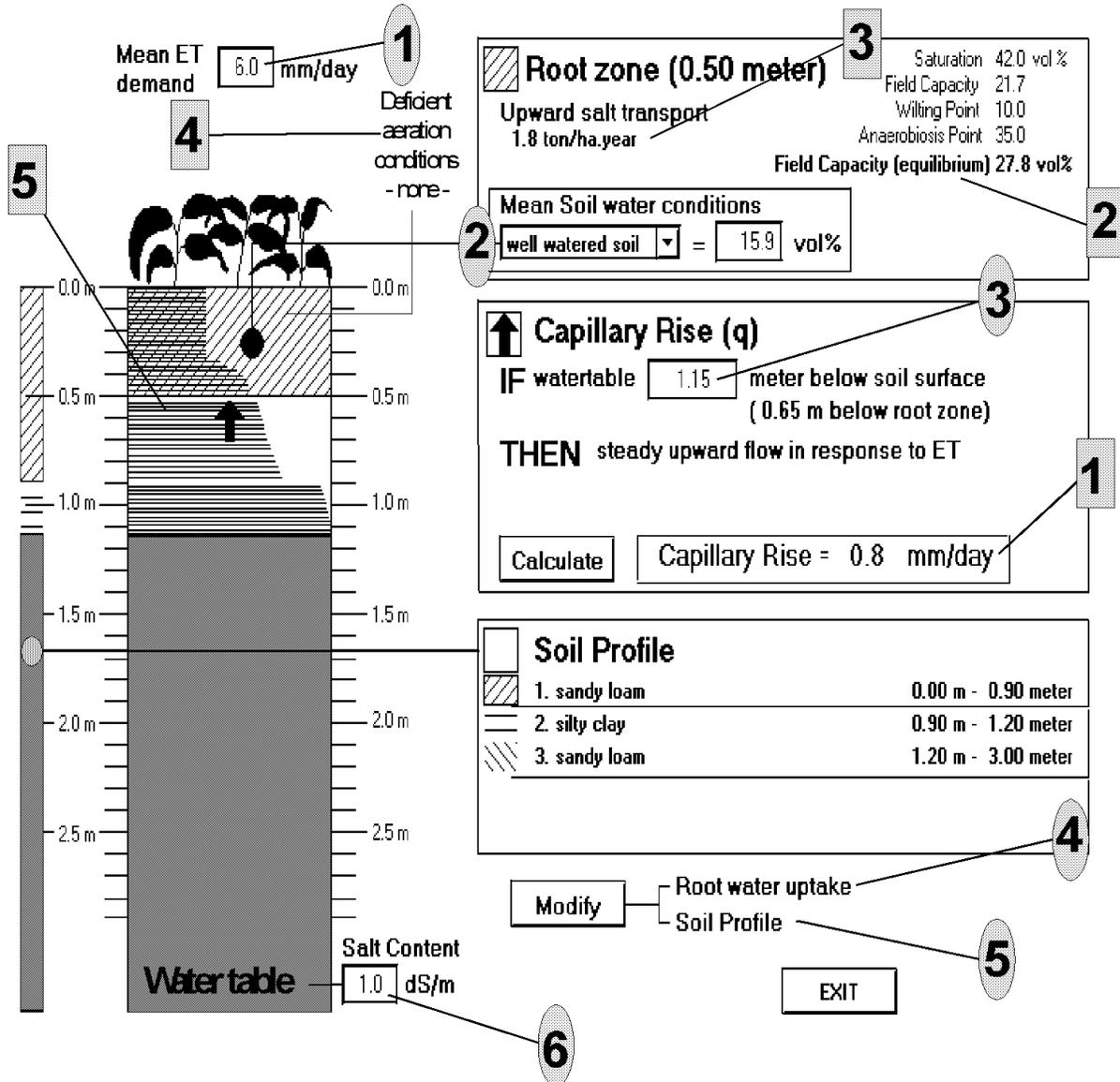
requirement. With UPFLOW the capillary rise was estimated for the given environmental conditions (Fig. 2) and the results were integrated in the irrigation charts for Mango's (DIM et al., 2001).
