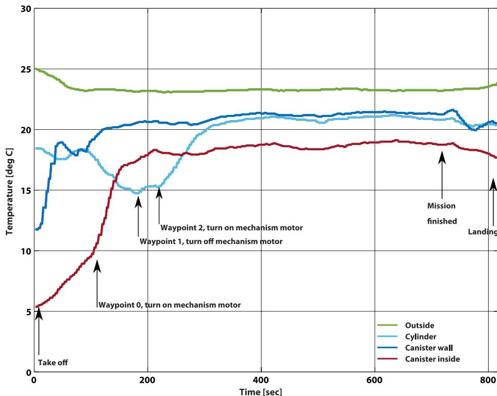
**Fig. 4. Dynamics of the temperature inside the release system during a flight.** The flight altitude was 100 m and corresponds to the line release of 21 March 2018 described in Table 1.
