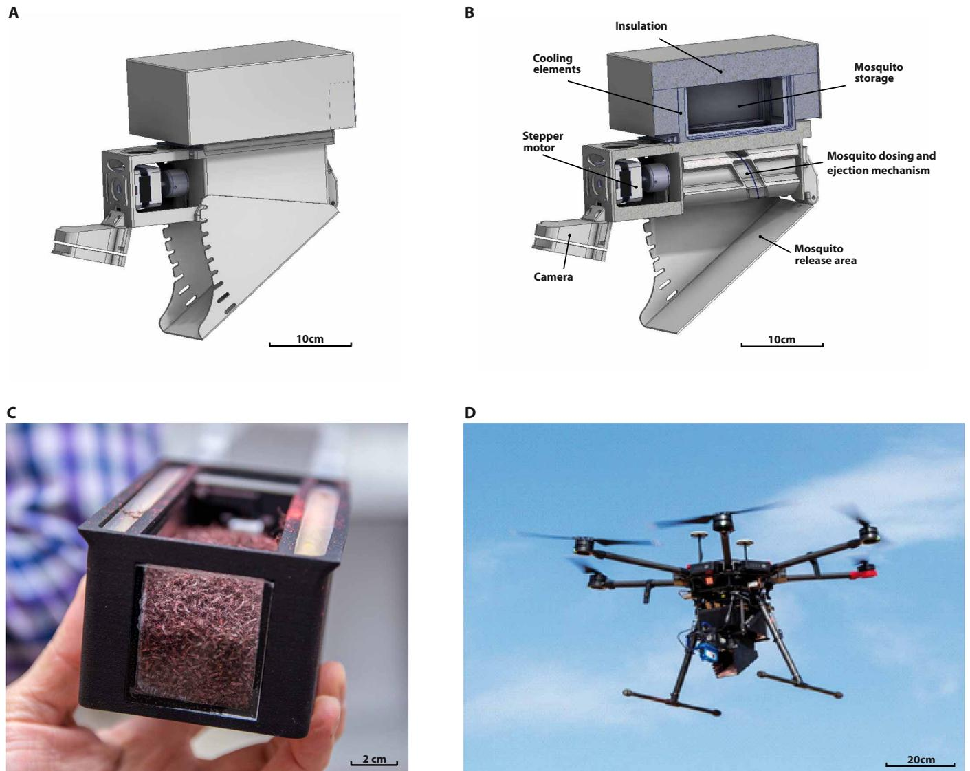
**Fig. 1. The adult mosquito release system operated from an UAV. (A)** Front right view of the release mechanism (technical drawing). **(B)** Half-section of the release mechanism (technical drawing). **(C)** Canister filled with 50,000 marked mosquitoes. **(D)** Fully assembled aerial mosquito release system attached to a DJI M600 UAV in flight.
